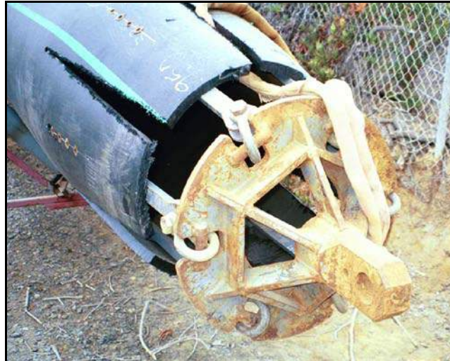
Figure 173. —A nose cone configuration utilizing a pull ring.
