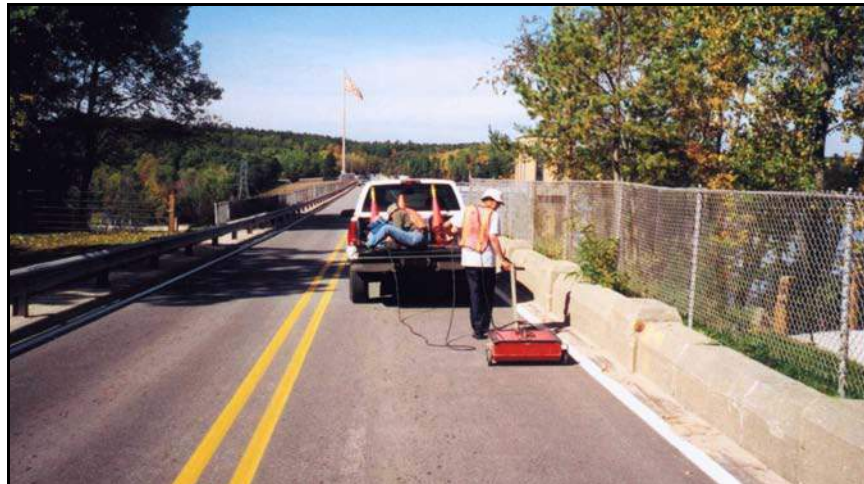
Figure 142. —Conducting a ground-penetrating radar survey across dam crest to locate voids beneath roadway and spillway. Photo courtesy Schnabel Engineering.
