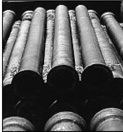
Figure 30. —Cast iron pipe is not considered acceptable for use in conduit applications.
