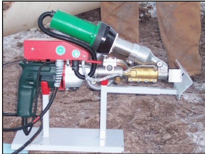
Figure 167.—Hand held extrusion gun.
