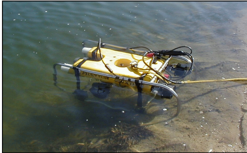
Figure 125. —An observation-class ROV entering the water to begin an inspection.
