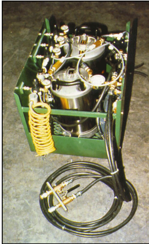
Figure 196. —An example of resin injection equipment used for small repair projects. Components are pumped independently and mixed at the nozzle for injection.
