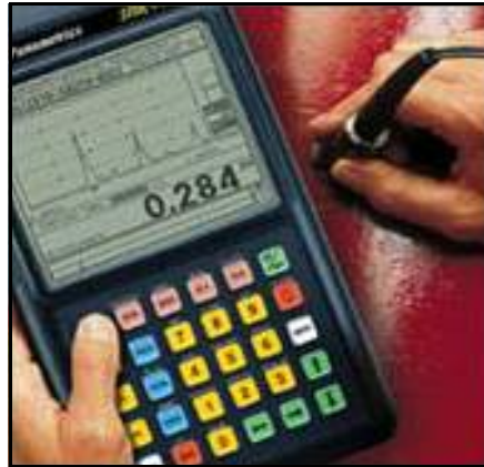
Figure 146. —Ultrasonic thickness gauge for measuring metal thickness.
