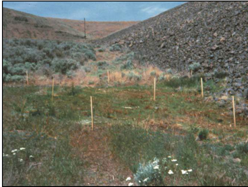
Figure 137. —The perimeter of a wet area at the downstream toe of an embankment dam located with wooden stakes.
