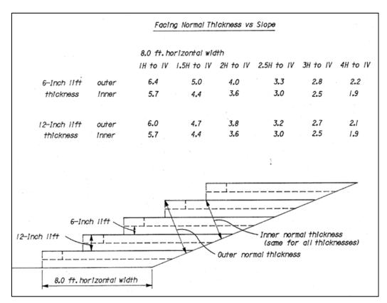
Figure 17.5.4-1. Soil-cement normal thickness at various slopes.
