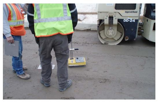
Figure 17.6.6.3-1. Use of nuclear gage to determine in-place density at Warren H. Brock Reservoir, California.
