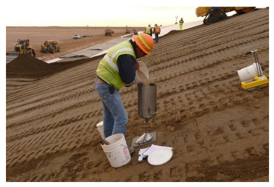
Figure 17.6.6.3-2. Use of sand-cone method to determine in-place density at Warren H. Brock Reservoir, California.
