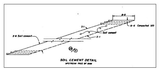
Figure 17.5.3-1. Typical stairstep soil-cement configuration.
