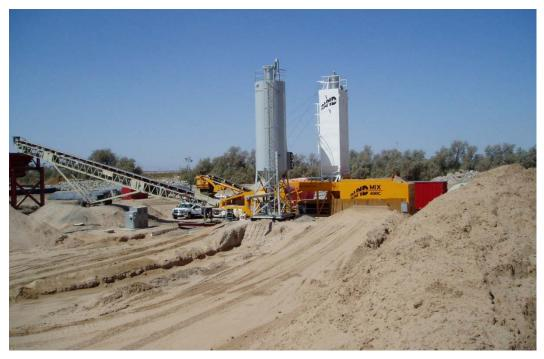
Figure 17.6.2-1. Pugmill used to make soil-cement at Warren H. Brock Reservoir, California.
