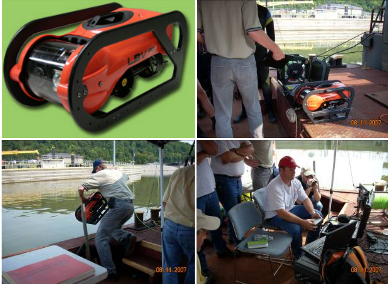
Figure A3. SeaBotix system showing (clockwise from upper left): LBV150SE ROV with color camera, black and white camera, and light mounted on tilt frame behind front cylindrical window; ROV with underside skid-mounted BlueView sonar, topside control/display unit, and tether reel; Scott Kinzel piloting ROV patiently and well; one-person deployment/recovery.
