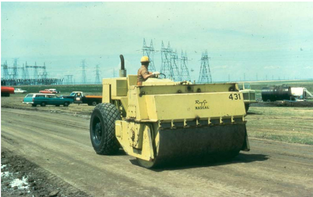
Figure 10.6.1.1-4 Vibratory, smooth drum, steel-wheeled roller. Good for rolling gravel and rock fill.
