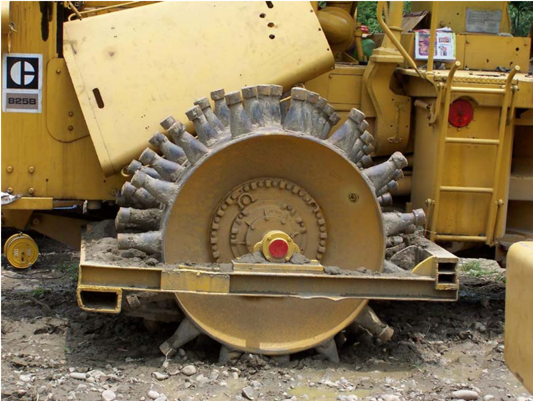
Figure 10.6.1.1-1 Carrion toothed roller, which is similar to a sheepsfoot or tamping type roller. These type rollers are generally used in more clayey or plastic soils.
