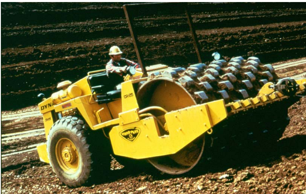
Figure 10.6.1.1-2 Vibratory, padfoot roller. These type rollers are generally used in more silty soils.
