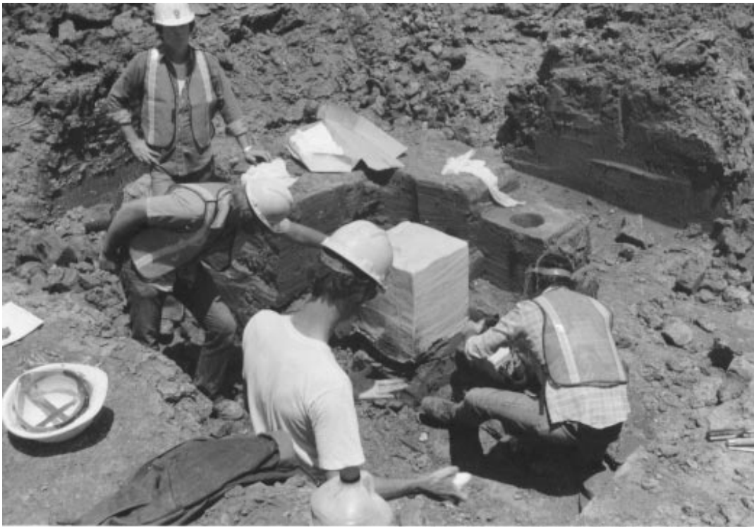
Figure 10.6.3.5.2-1 McPhee Dam, Colorado. Block sample from test pit in zone 1. Final saw cut is being made beneath the sample using a chain saw equipped with special tungsten carbide teeth. Also visible is an area where an in-place density test was taken 2 feet upstream of the block sample, 1983.
