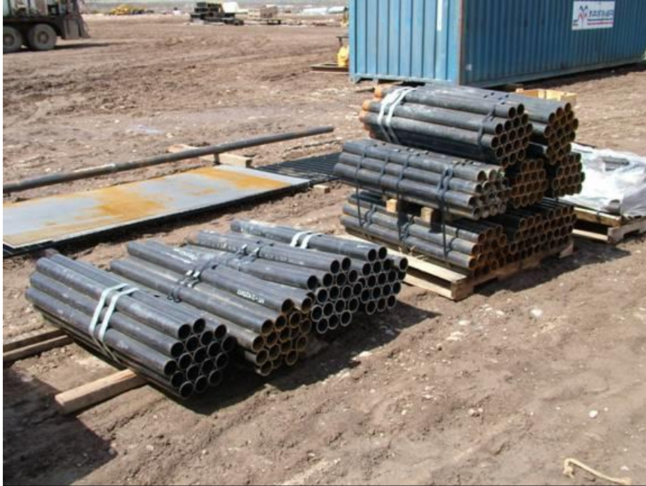
Figure 15.12.12-1. Standpipes used for a recent Reclamation project.
