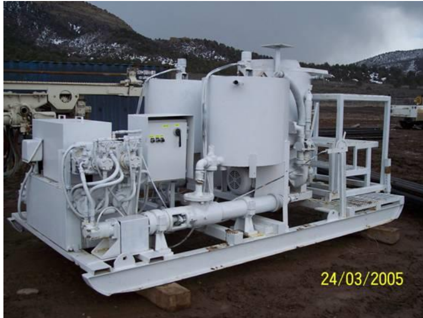
Figure 15.12-2. Portable batch plant at Ridges Basin Dam.
