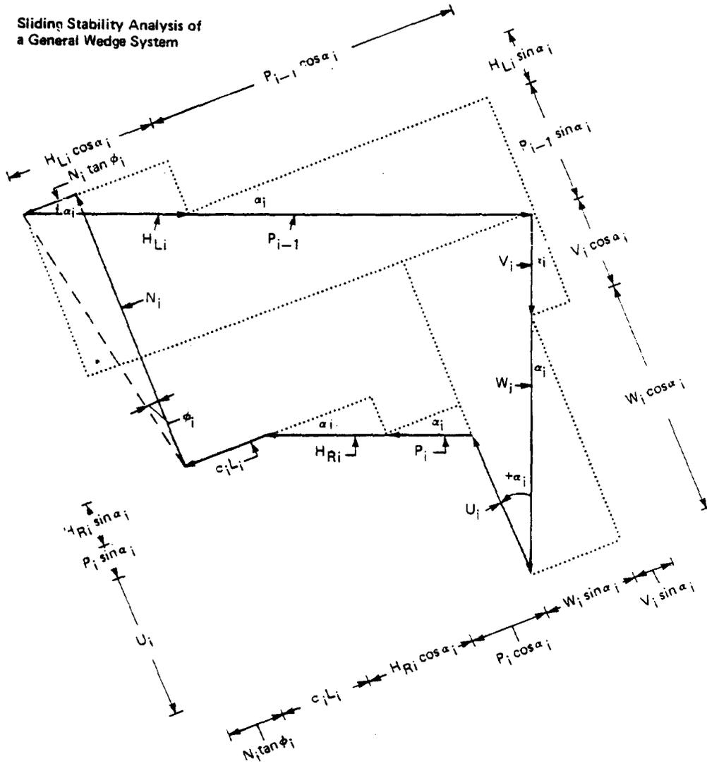
A sliding stability analysis using the general wedge equation should yield results comparable to those obtained from graphical solutions using force polygons. This is clarified by the following discussion of the force polygon shown above
