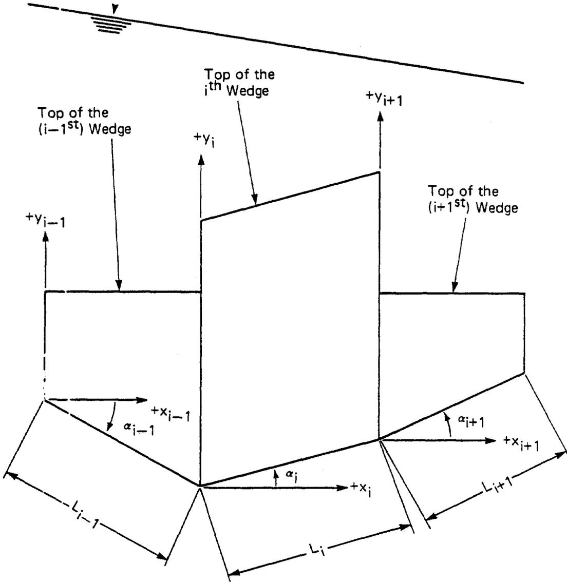
Figure 2. Geometry of the Typical  $i$ th Wedge and Adjacent Wedges
