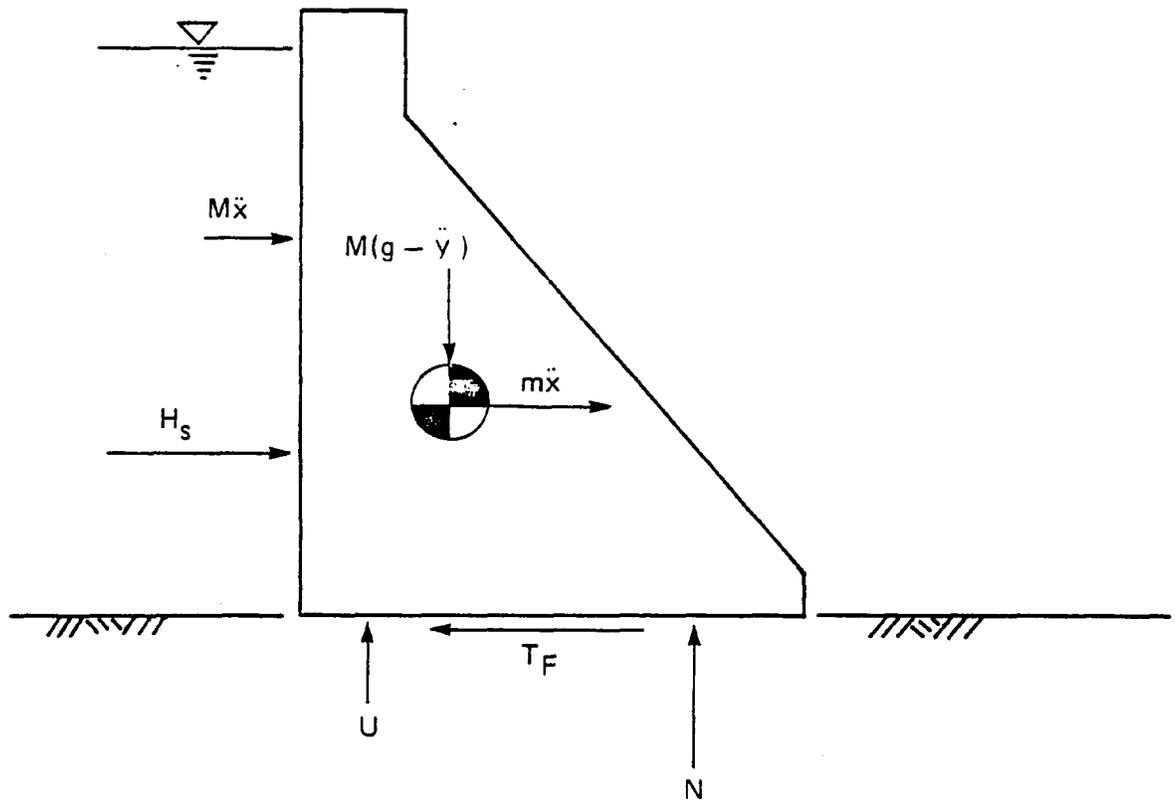
Figure 11. Seismically Loaded Gravity Dam
