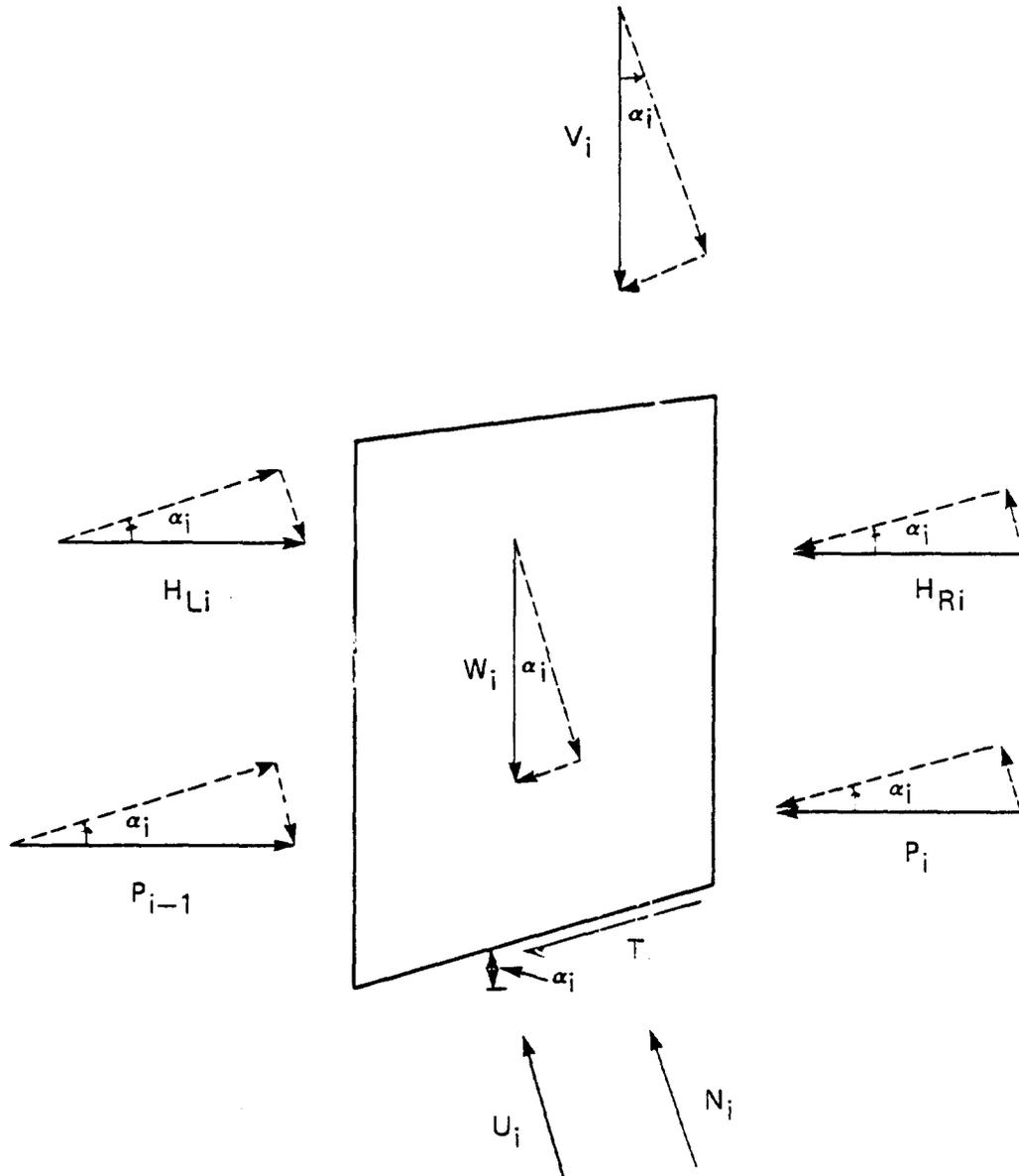
Figure 4. Free Body Diagram of the  $i^{\text{th}}$  Wedge
