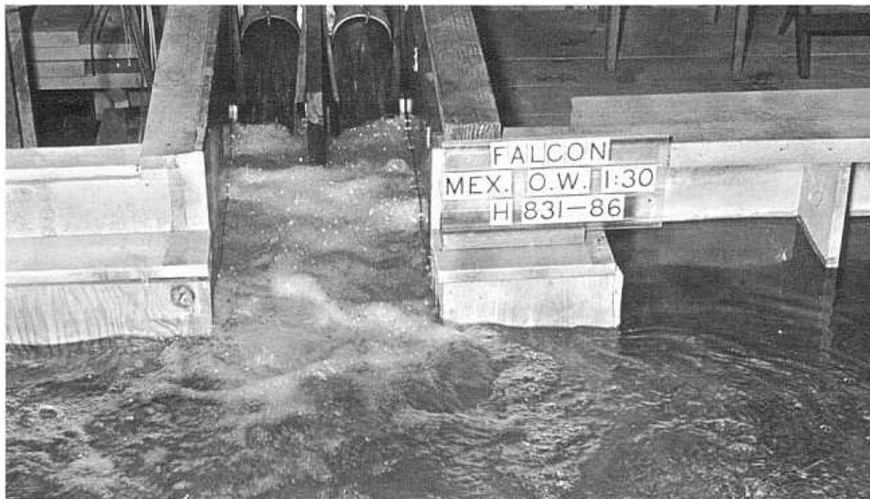
90-inch valves fully open, discharging 4,570 c.f.s. Reservoir elevation 300, approx. Tail water elevation 181.2.
