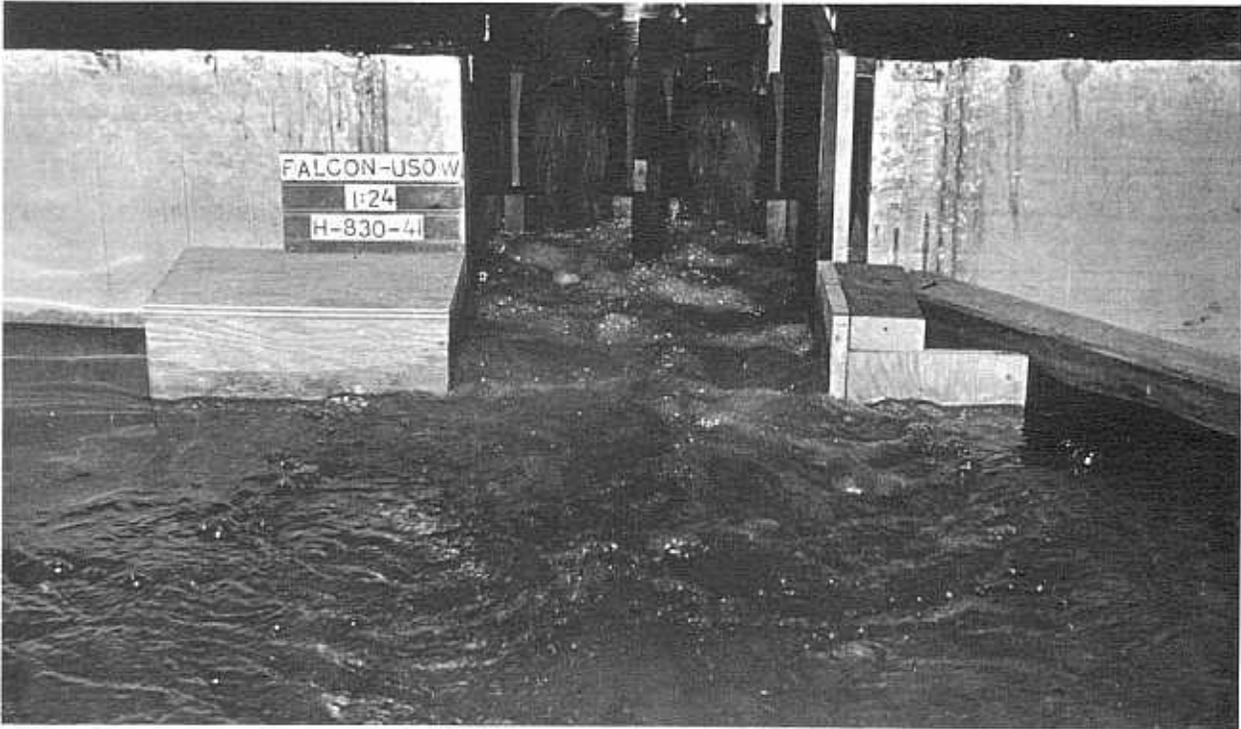
72-inch valves fully open, discharging 2,920 c.f.s. Reservoir elevation 310, approx. Tail water elevation 180.8.
