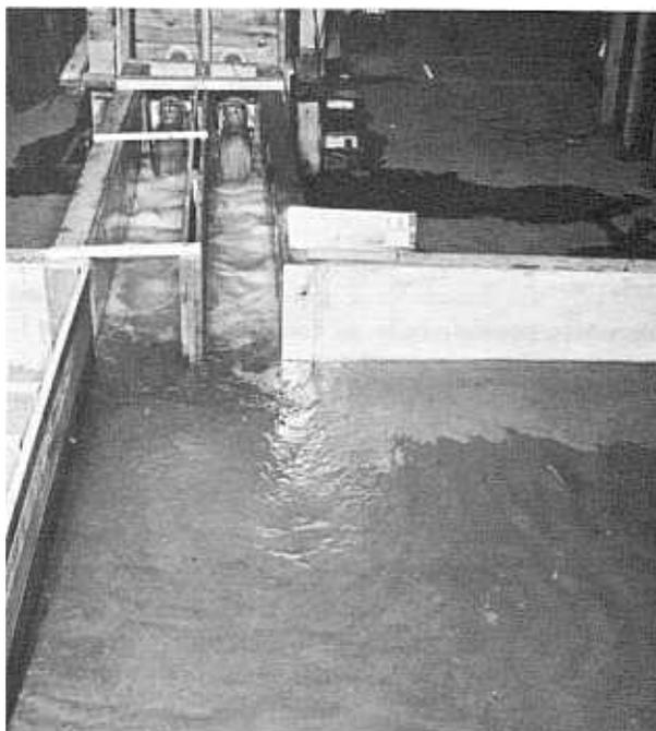
FIGURE 90.—Boysen Dam: outlet works discharging 1,320 c.f.s.—model scale: 1:16.
