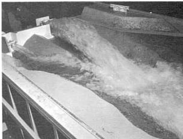
FIGURE 156.—*Tube elbow bucket produces clear-cut stable jet with little spray. Discharge 28,650 c.f.s. maximum.*
