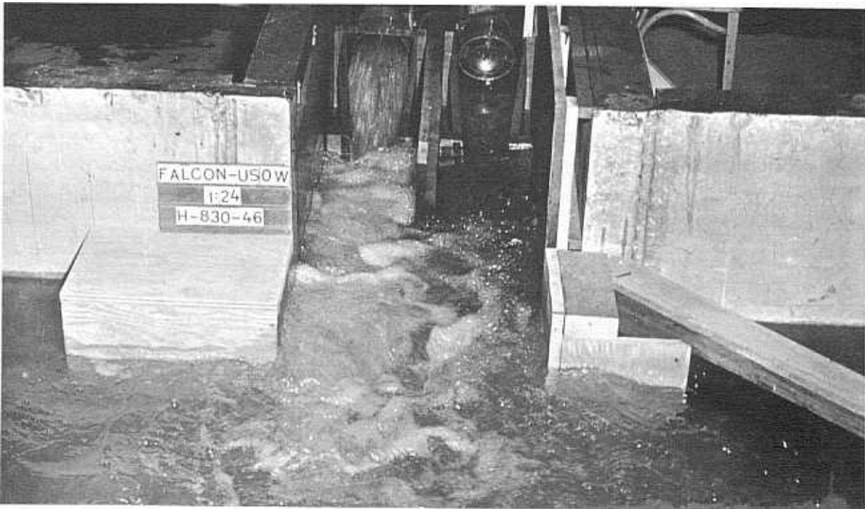
72-inch right valve fully open, discharging 1,600 c.f.s. Reservoir elevation 310, approx. Tail water elevation 180.5.
