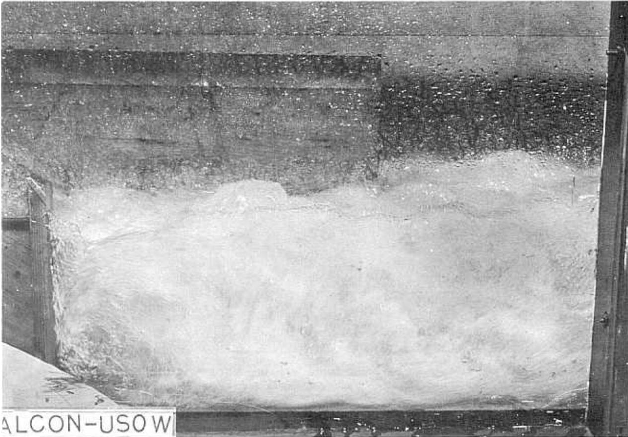
72-inch valves open 100%, discharging 2,920 c.f.s. Reservoir elevation 310, approx. Tail water elevation 180.8.
