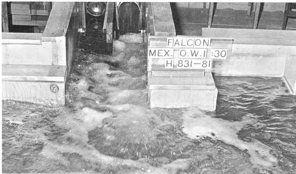
90-inch left valve fully open, discharging 2,400 c.f.s. Reservoir elevation 300, approx. Tail water elevation 181.2.
