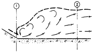
Type I – Hydraulic jump, horizontal apron
