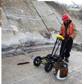
Reclamation Dam – Void below spillway chute floor; ground penetrating radar (GPR) identifying voids; and spillway chute foundation and floor replacement to mitigate foundation piping and high potential of stagnation pressure failure
