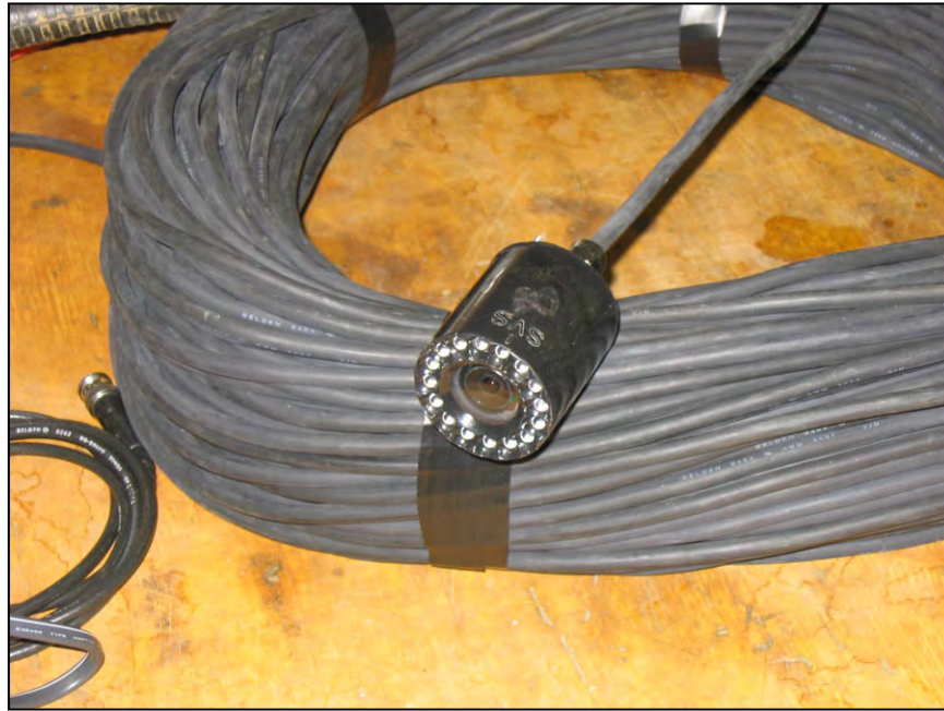
Figure 161. —Small video camera that can be attached to PVC or metal poles and manually pushed into underdrain pipes.
