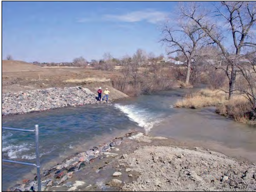
Figure A-99.—View looking downstream at the outfall channel during testing of one of the fixed-cone valves at 35 percent opening ( 147 \text{ ft}^3/\text{s} ).
