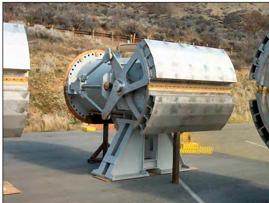
Figure 108.—48-inch diameter clamshell gate before installation.
