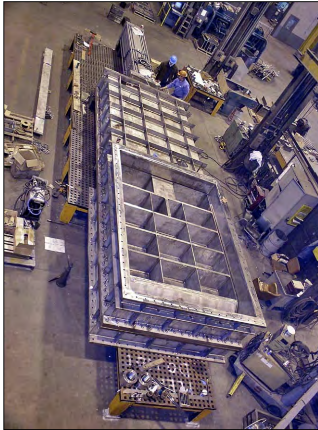
Figure 102.—A fabricated (stainless steel) bonneted gate being produced for 200 feet of head. Photo courtesy of Rodney Hunt Corporation.
