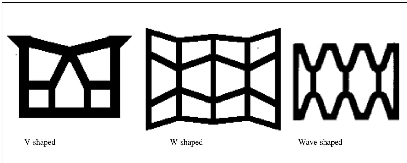
**Figure 3-3. Preformed compression seals are compartmentalized in their internal structure for compressible behavior. Shown are three of the several types and shapes of preformed compression seals available as stock materials**
