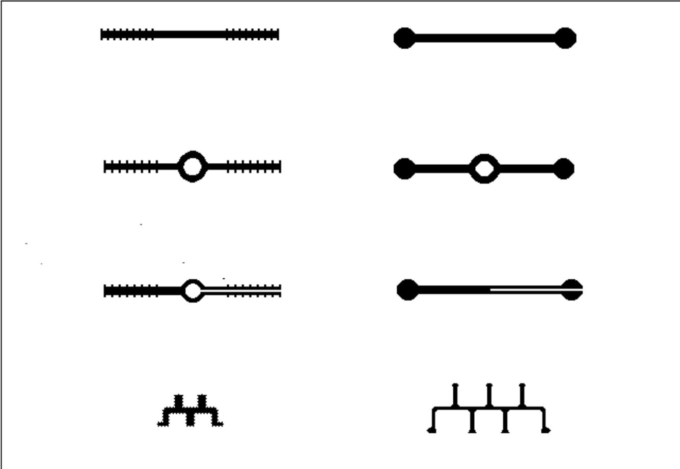
Figure 3-1. Various types and shapes of nonmetallic waterstops
