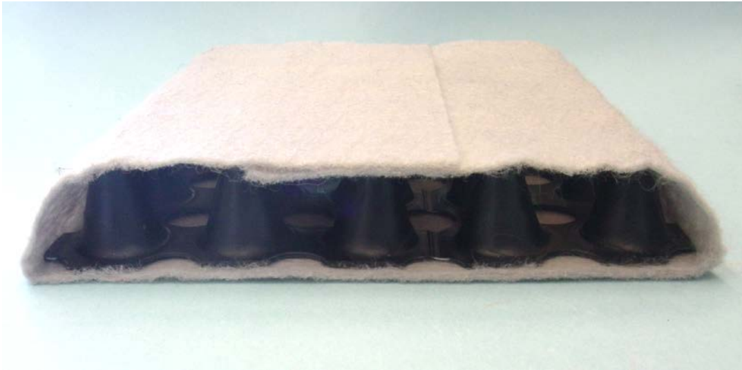
Figure 2.16.—Photograph of a geocomposite edge drain made by wrapping a geotextile tube around a vacuum-formed drainage core.
