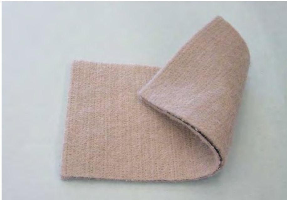
Figure 2.12.—A double-sided geocomposite geomembrane made by bonding geotextiles to both sides of a geomembrane (black colored core).
