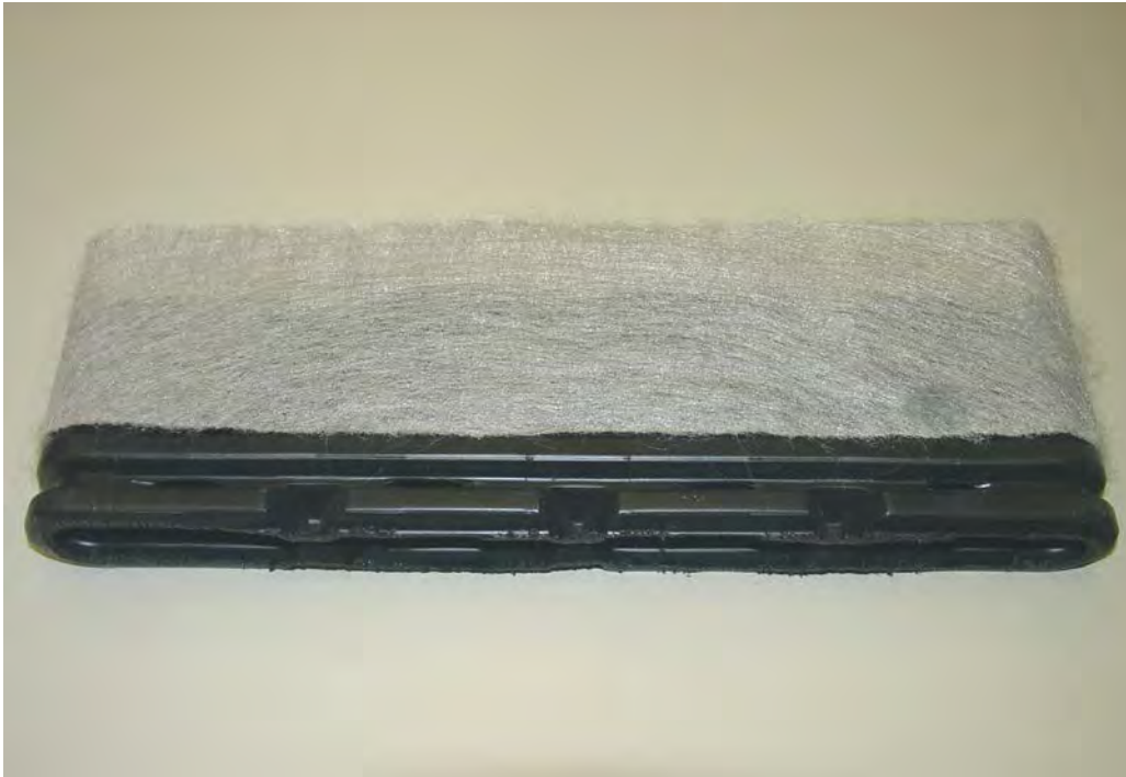
Figure 2.18.—Photograph of a geocomposite edge drain made by placing a perforated geosynthetic core inside a geotextile tube. The core functions as a flat-shaped pipe.
