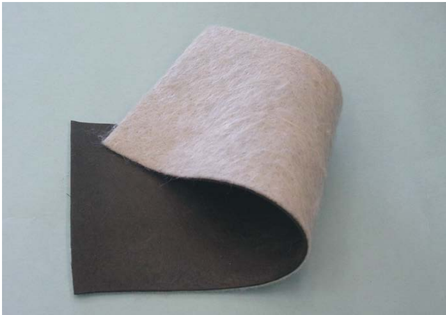
Figure 2.11.—Photograph of a single-sided geocomposite geomembrane. It is made by bonding a geotextile (grey colored layer) to one side of a geomembrane.
