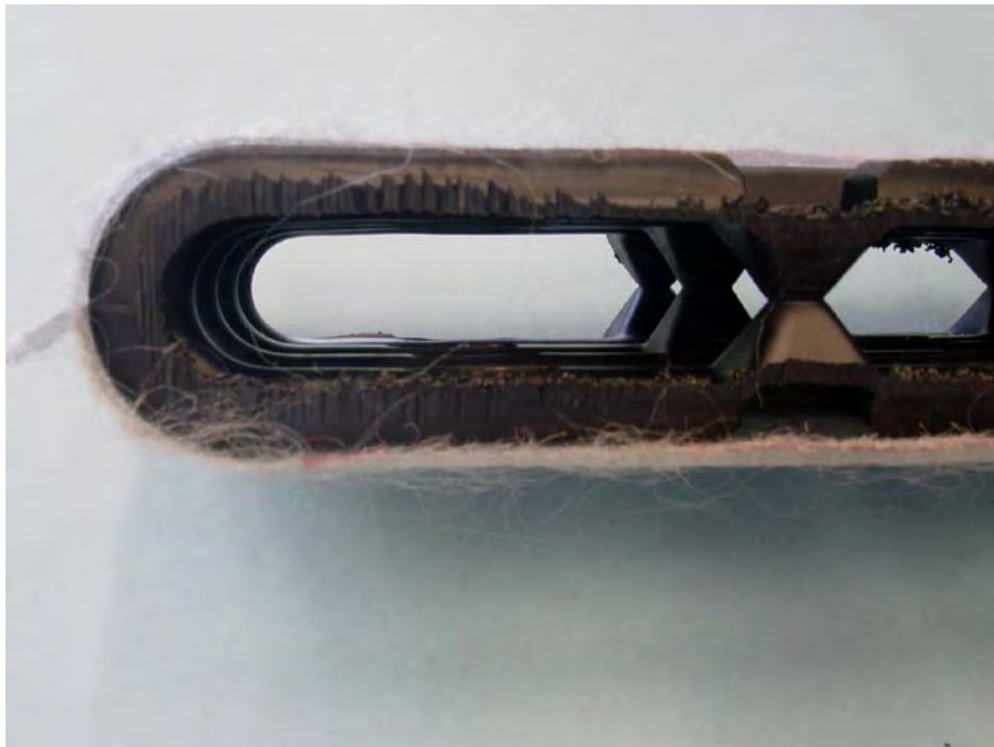
Figure 2.19.—Photograph showing a close-up view of a portion of the geocomposite drain shown in figure 2.18.
