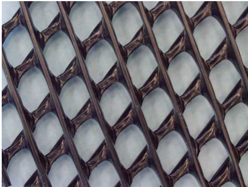
Figure 2.7.—Photograph of a bi-planar geonet. It is made from two layers of polymeric strands or ribs.
