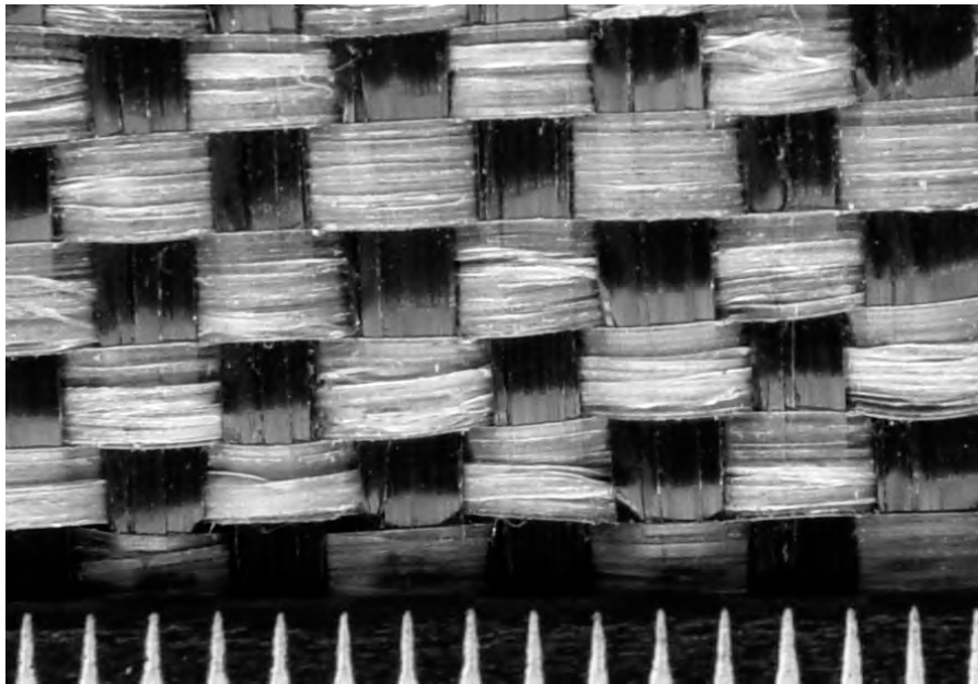
Figure 2.26.—Woven slit film geotextile, magnified view (1 mm scale).
