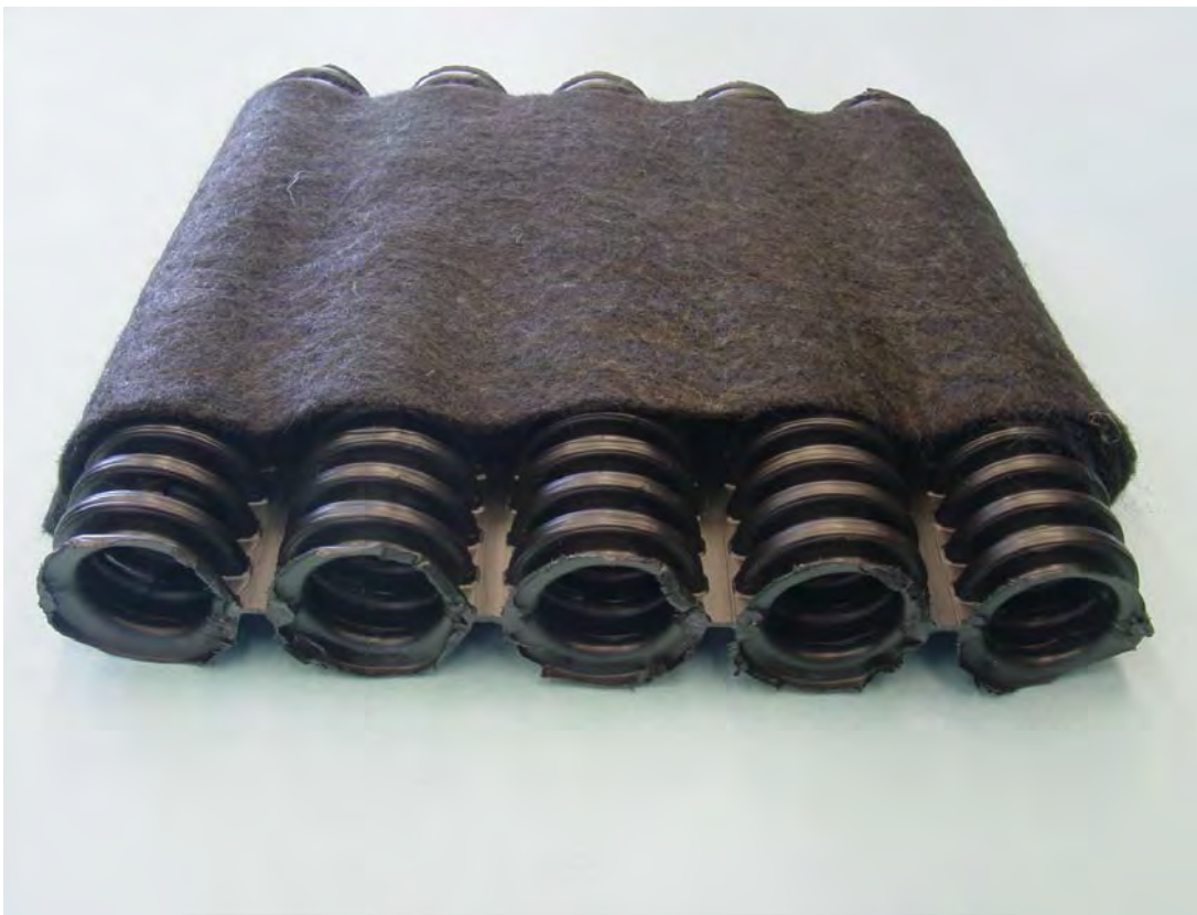
Figure 2.17.—Photograph of a geocomposite drain formed by enclosing a row of perforated geopipes inside a geotextile tube.
