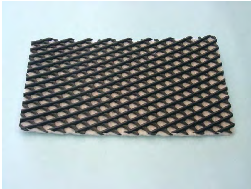
Figure 2.9.—Photograph of a single-sided bi-planar geocomposite geonet composite. It is made by bonding a geotextile to one side of a geonet.
