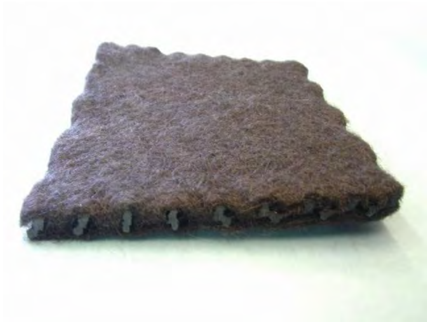
Figure 2.13.—Photograph of a geocomposite geonet drain made by bonding a geotextile to each side of a bi-planar geonet.
