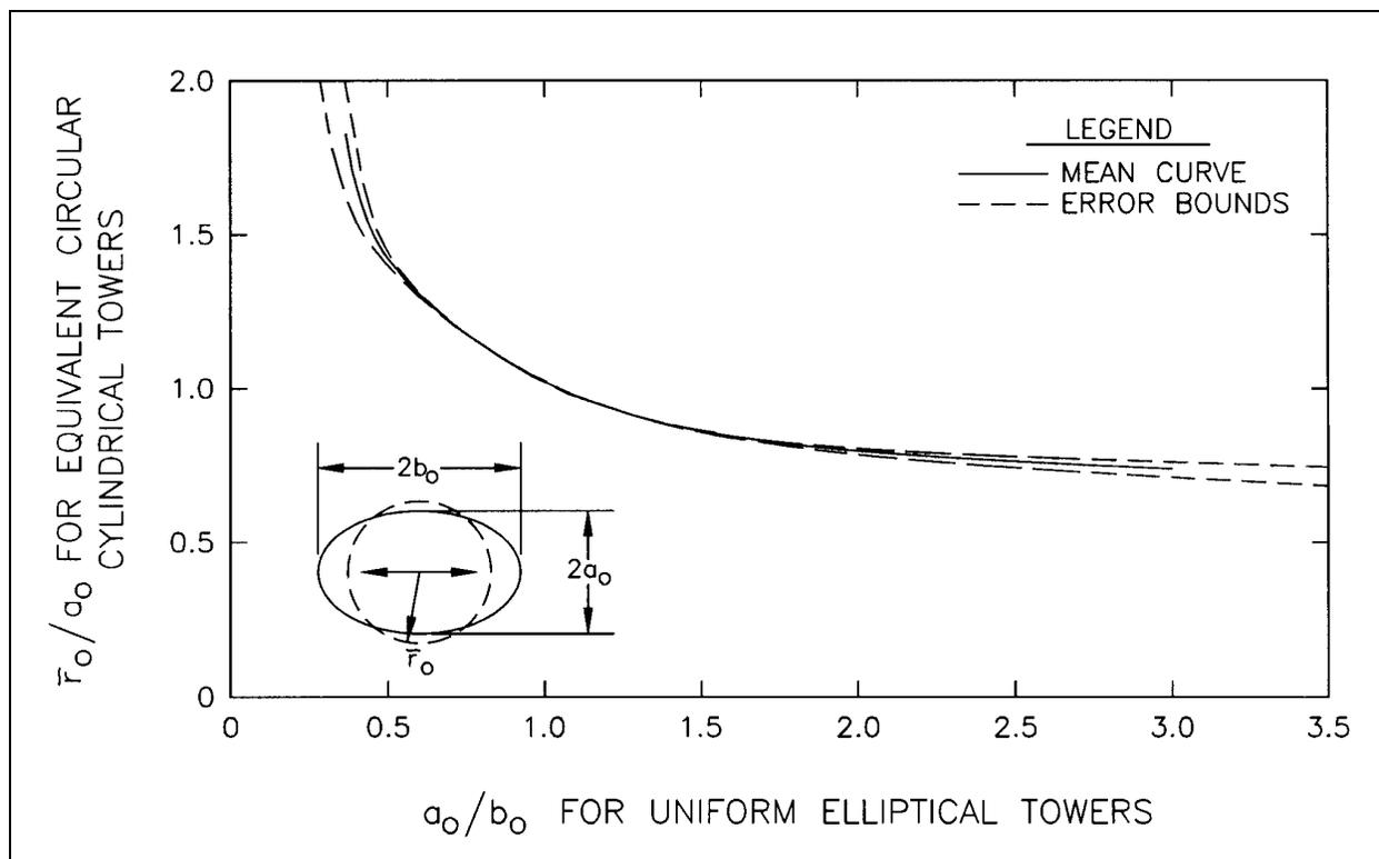
Figure D-4. Equivalent radius of circular towers for outside hydrodynamic added mass
