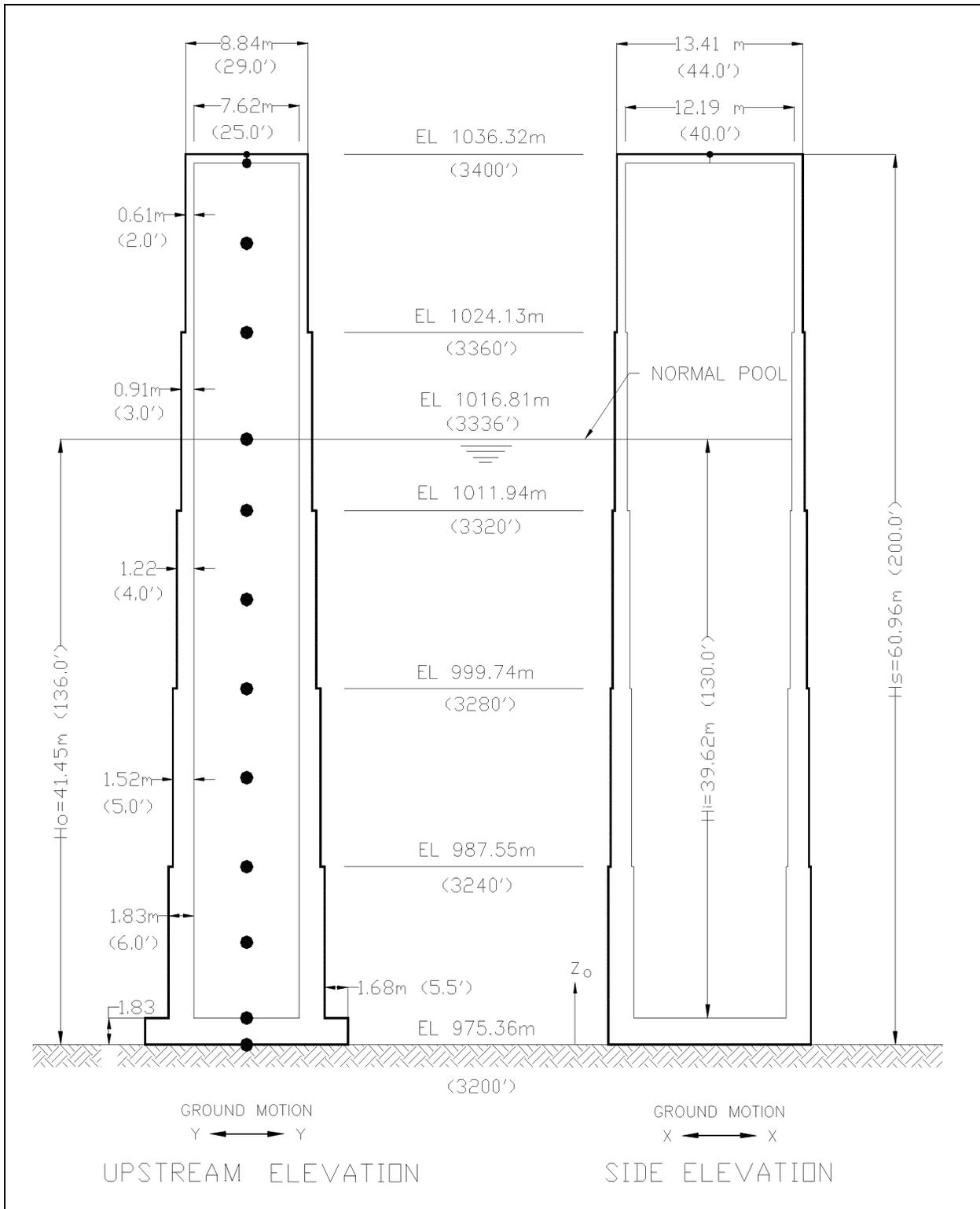
Figure C-1. Tower geometry
