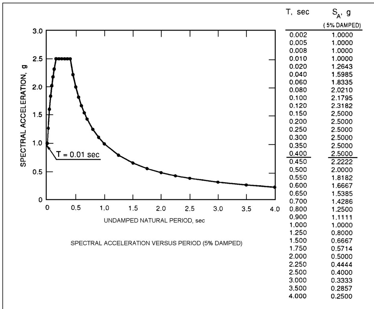
Figure C-12. Response spectrum seismic input for computer analysis
