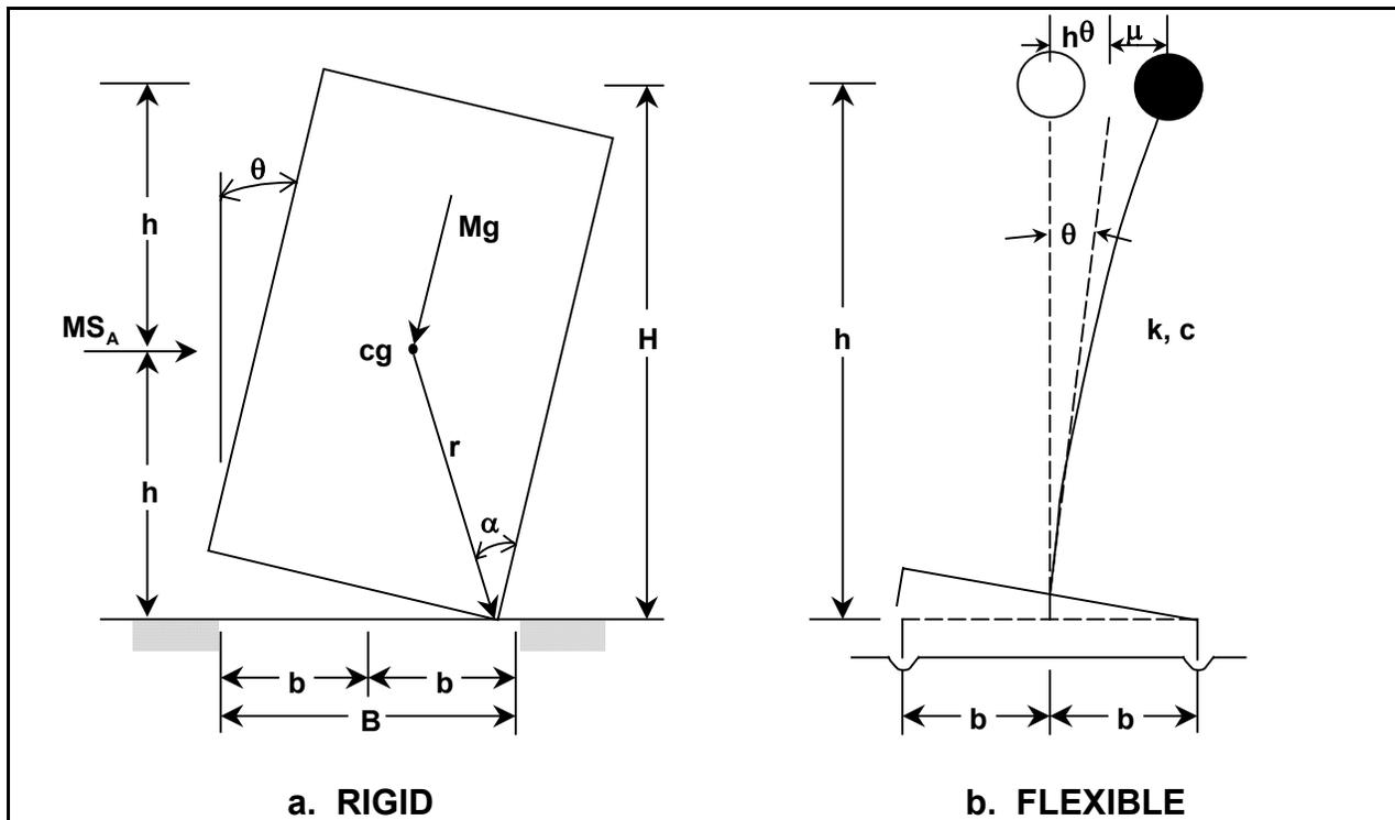
Figure E-1. Rigid block and SDOF models for dynamic rotational stability (where  $c$  = damping coefficient for the structure;  $\theta$  = rigid body rotational degree of freedom;  $\mu$  = flexural deflection of the top of the structure; and  $k$  = stiffness of the structure)
