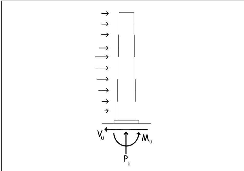
Figure C-17. Loads acting on tower during an earthquake
