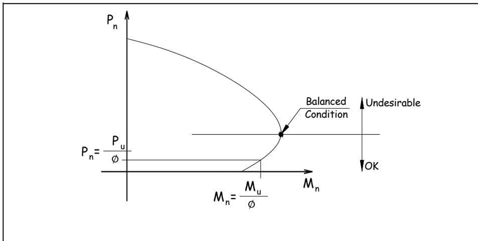
Figure C-18. Axial force and bending moment interaction diagram
