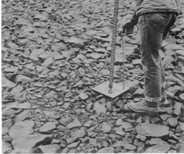
Figure 11-2. Apparatus for taking level readings
