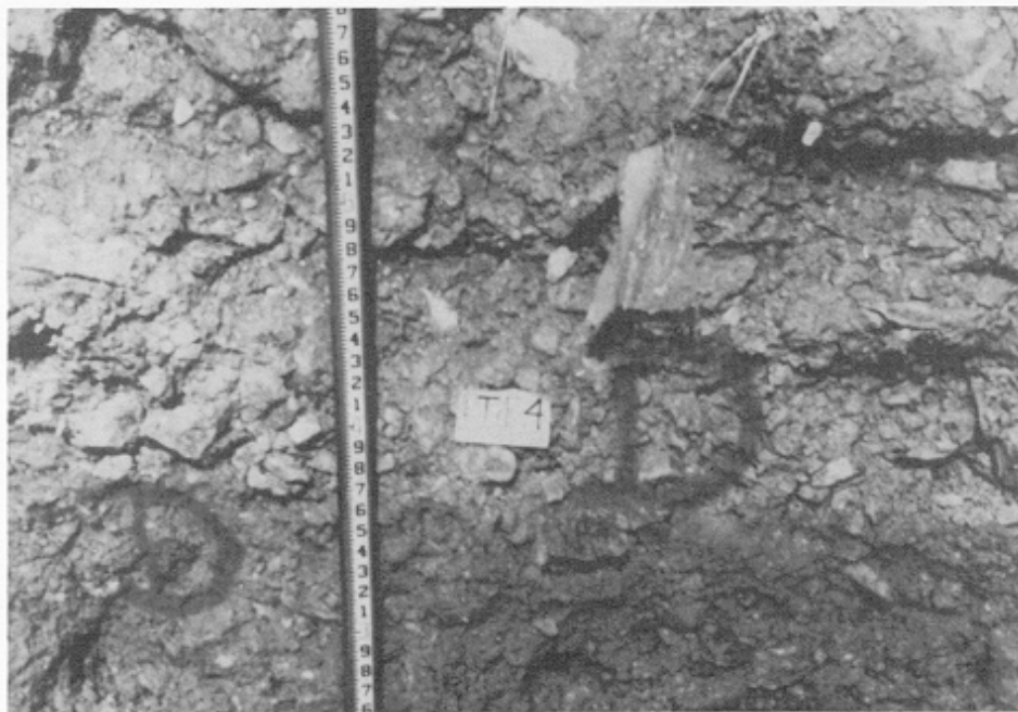
Figure 12-21. Photographs of rockfill containing appreciable fines, Cerrillos Dam test fill No. 4 inspection trench
