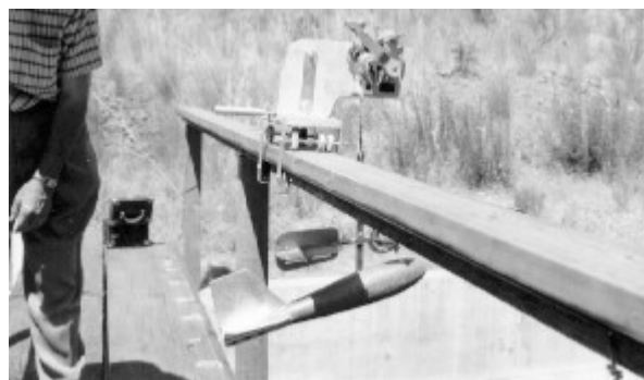
Figure 10-7 -- Carriage and track for handling current meter and weights from a bridge. A 2- by 6-in timber permanently attached to the bridge rail is the track for the portable, wheeled carriage that supports the reel, cable, and meter assembly.
