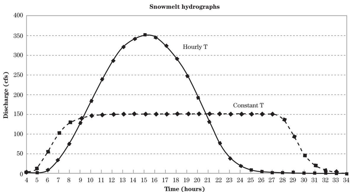
**Note:** This plot was calculated using HEC-1 with the runoff data from example 11-4 above.
