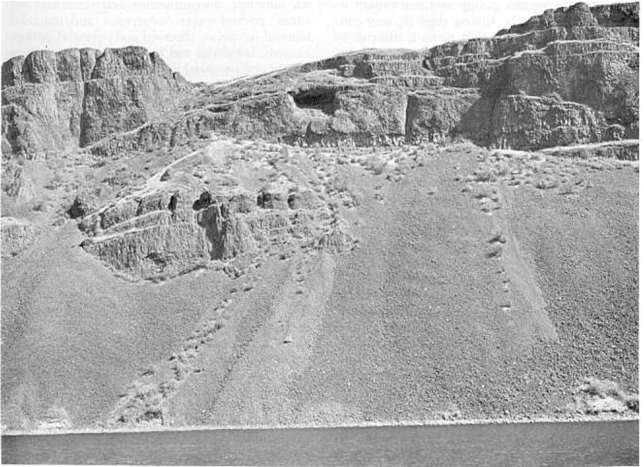
Figure 5-3.—Typical talus deposit suitable for riprap. At base of basalt cliffs in Grant County, Washington. 3PPG-1.
