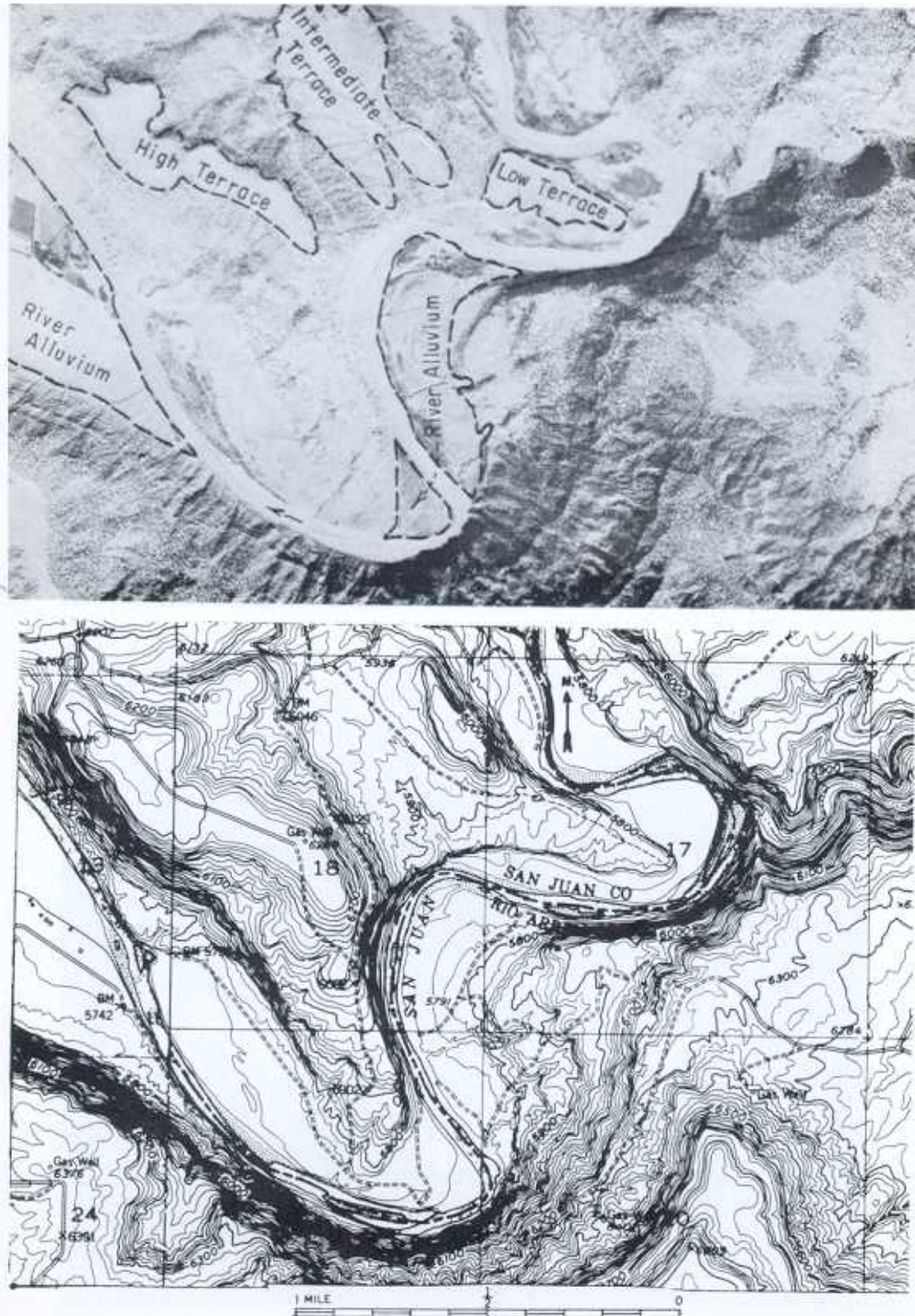
Figure 5-29.—Aerial view and topography of stream deposit showing river alluvium and three levels of gravel terraces. (Photograph by USGS). PX-D-16259.
