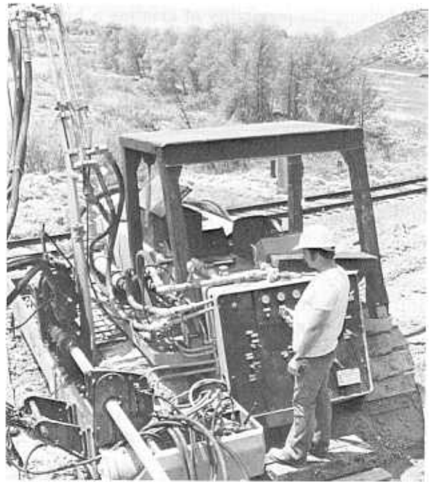
Figure 5-51.—Horizontal rotary drill. Aardvark Model 500 drill with adjustable box-beam slide, crawler-tractor mounted. P126-100-4001.
