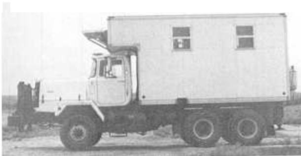
Figure 5-40.—Self-contained, truck-mounted, electrical cone-penetration apparatus.
