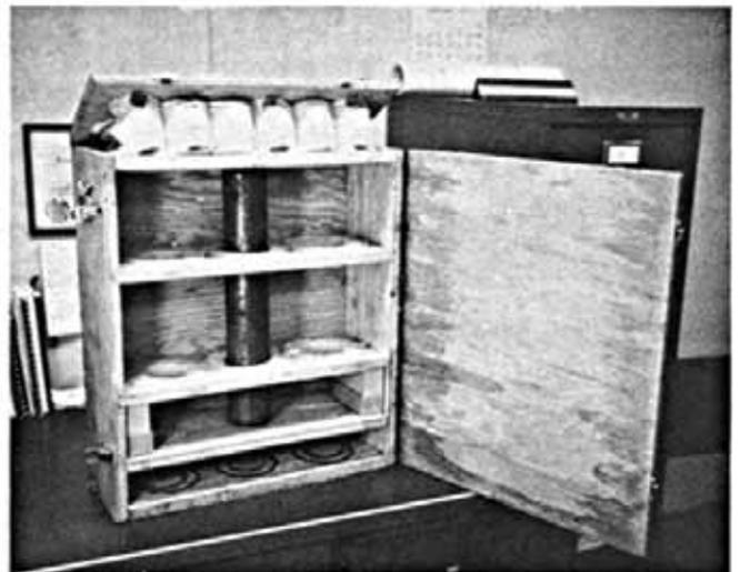
Sample tube supported vertically by spring action and laterally by shaped, rubber-padded inserts.
