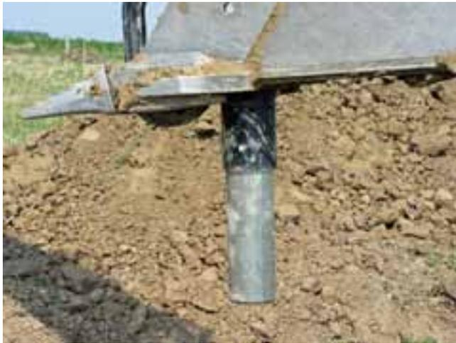
**Figure 5-3** Thin-wall open-drive sampler
