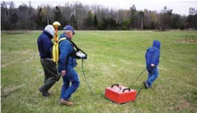
(c) Portable electromagnetic imaging tool (Geonics EM–34)
